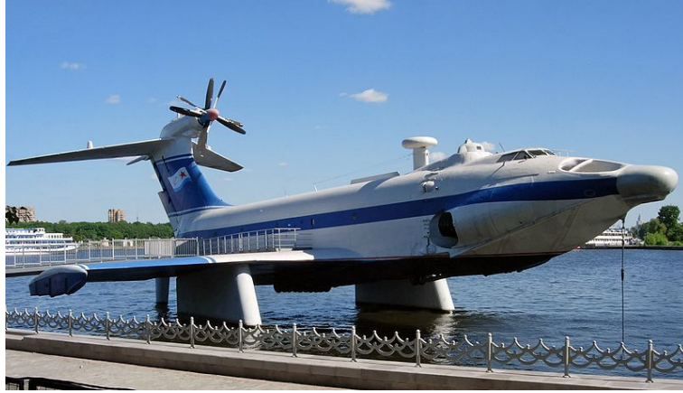
Figure 1.1: Soviet Ekranoplan, a ground effect vehicle that flies a few meters above the surface[1]
